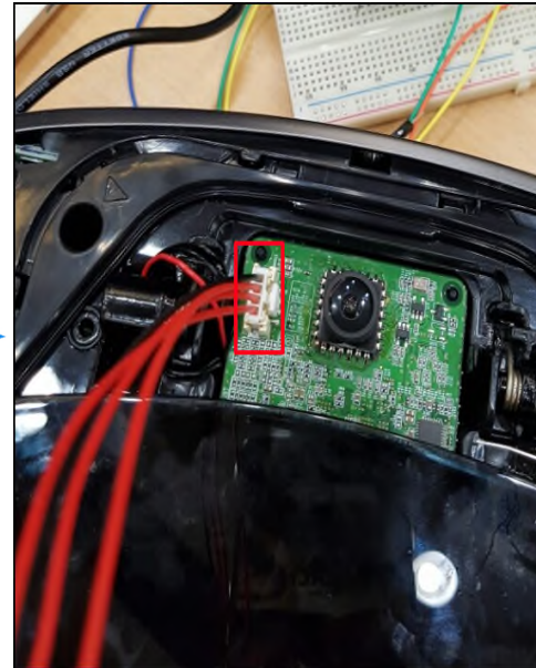
3. Identify UART pin (Vcc, Tx, Rx, Gnd)
