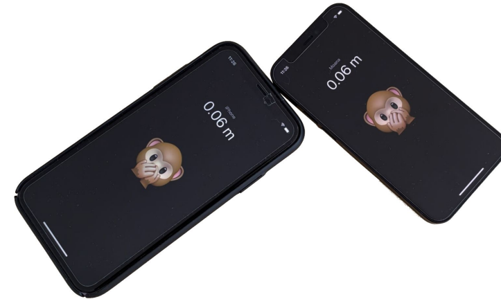
Nearby Interaction (iOS 14) Framework to enable ranging between Apple devices & third parties.
